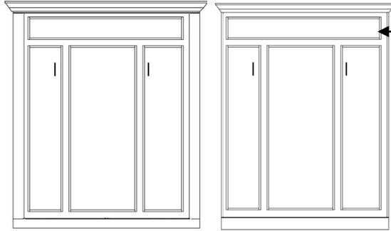
**TO OPEN**—WHEN YOU LIFT THIS PANEL FOOT YOU UNLATCH THE BED FROM THE CABINET TOP. ONCE PARTIALLY OPENED THE SAFE PISTON LIFT SYSTEM TAKES OVER AND THE BED SLOWLY LOWERS TO THE FLOOR
